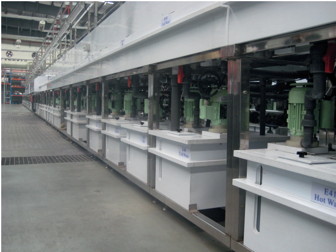
DO- Immersible pumps in galvanic process
