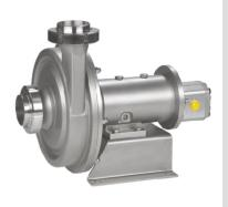
Stainless steel hygienic centrifugal pumps, which are used for pumping liquids up to 300 cP. Depending on the product to be pumped, the pumps can be supplied with a closed impeller, a half open impeller or an open impeller (suitable for pumping liquids with solids).
